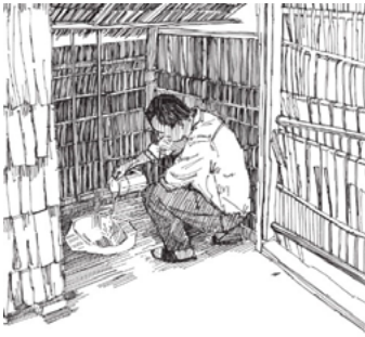
Figure 26. Flush to pit latrine
